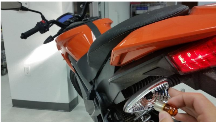
Figure 2: Pull out bulb and ensure front indicator begins to flash faster
