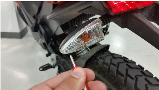
Figure 1: Removing indicator lens
