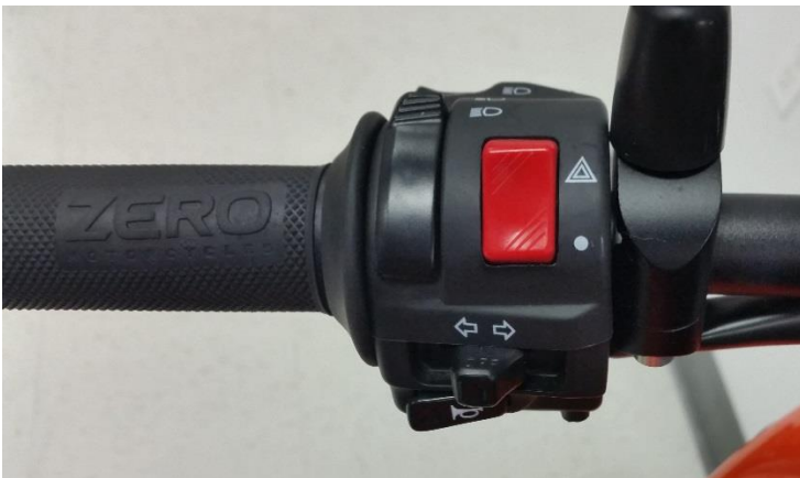
Figure 3: Red hazard switch to flash all four signal bulbs
