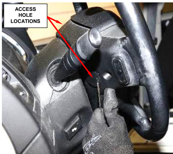
Figure 1 - DAB Screw Locations
