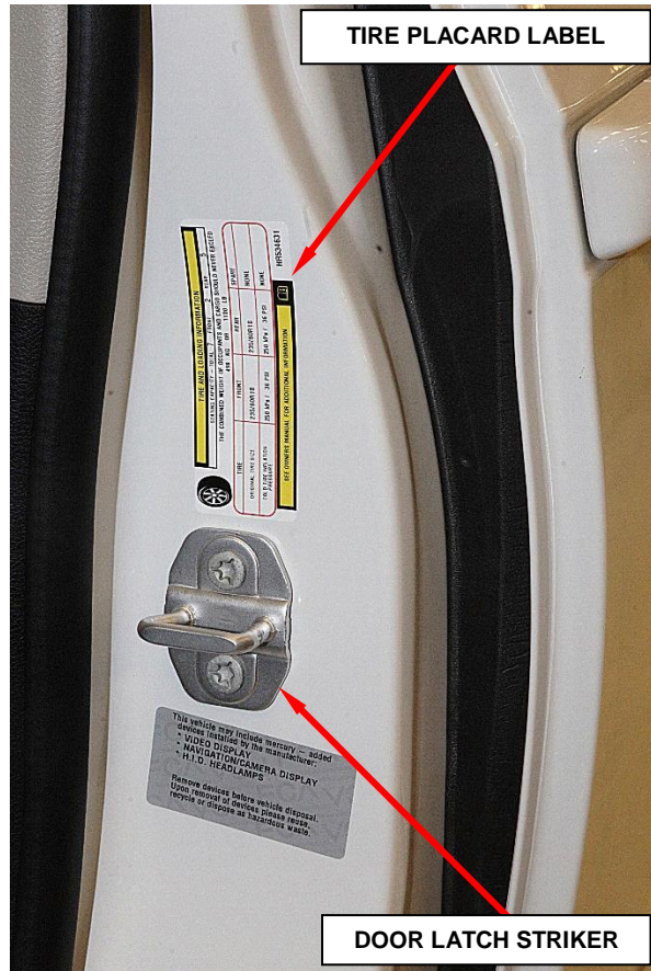
Figure 1 – Tire Placard Label Location
