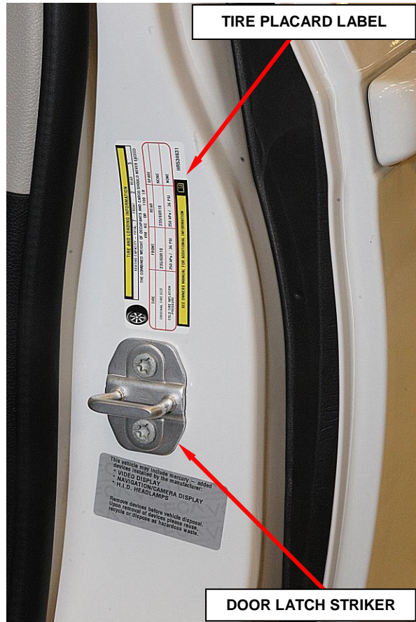
Figure 1 – Tire Placard Label Location
