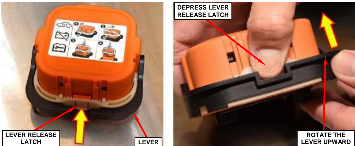
Figure 6 – High-Voltage Manual Service Disconnect First Stage Latch Release (High-Voltage Manual Service Disconnect Removed from Vehicle for Visual Clarity)
