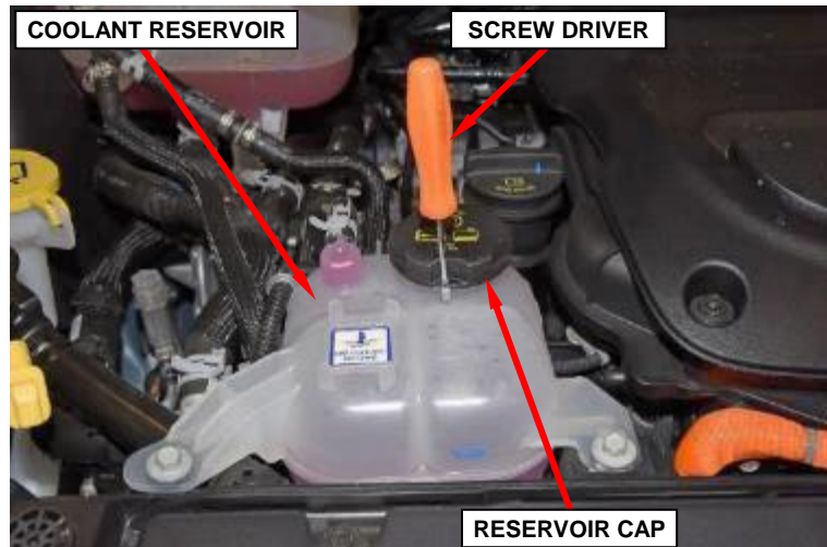
Figure 18 – Power Electronics Coolant Reservoir
