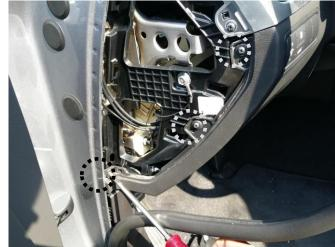
6. Remove crash pad lower panel mounting screw.
