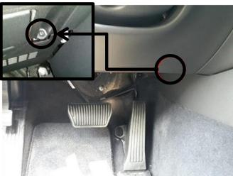
7. Separate the crash pad lower panel from the crash pad and then disconnect the two connectors.
