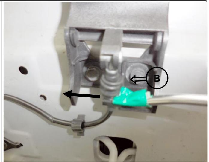
4. Rotate the cable upward, and then push the cable (C) to left to remove it from the release handle.
