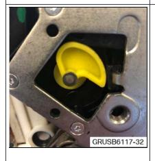
7. Manually position the cam so that it is clearly visible in the opening.
