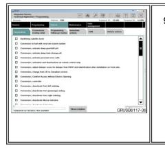
Select the conversion "Conversion, Comfort Access without Electric Opening" and program the vehicle with ISTA/P 3.63.3 (I-Level E065-17-11-520) or higher. The following K-Word will be added to the Vehicle Order: "CAOE"
