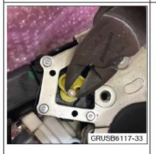
5. Cut the head of the cam retainer off with a pair of cutters.
