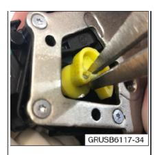
6. Slide the cam off and discard using a pair of needle nose vice grips.
