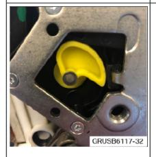
4. Manually position the cam so that it is clearly visible in the opening.
