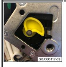
7. Manually position the cam so that it is clearly visible in the opening.
