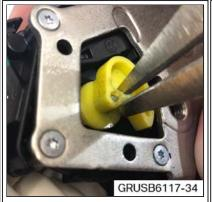
9. Slide the cam off and discard using a pair of needle nose vice grips.
