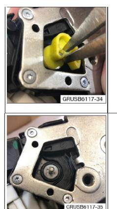
6. Slide the cam off and discard using a pair of needle nose vice grips.
