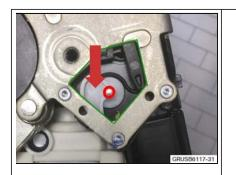
2. Once the door lock is removed, modify each lock by removing the white or yellow opening assist cam (red arrow).
