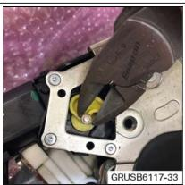
4. Cut the head of the cam retainer off with a pair of cutters.
