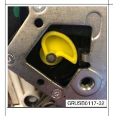
3. Manually position the cam so that it is clearly visible in the opening.
