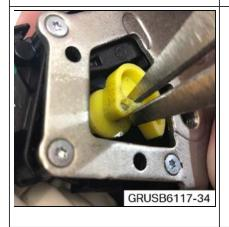
5. Slide the cam off and discard using a pair of needle nose vice grips.
