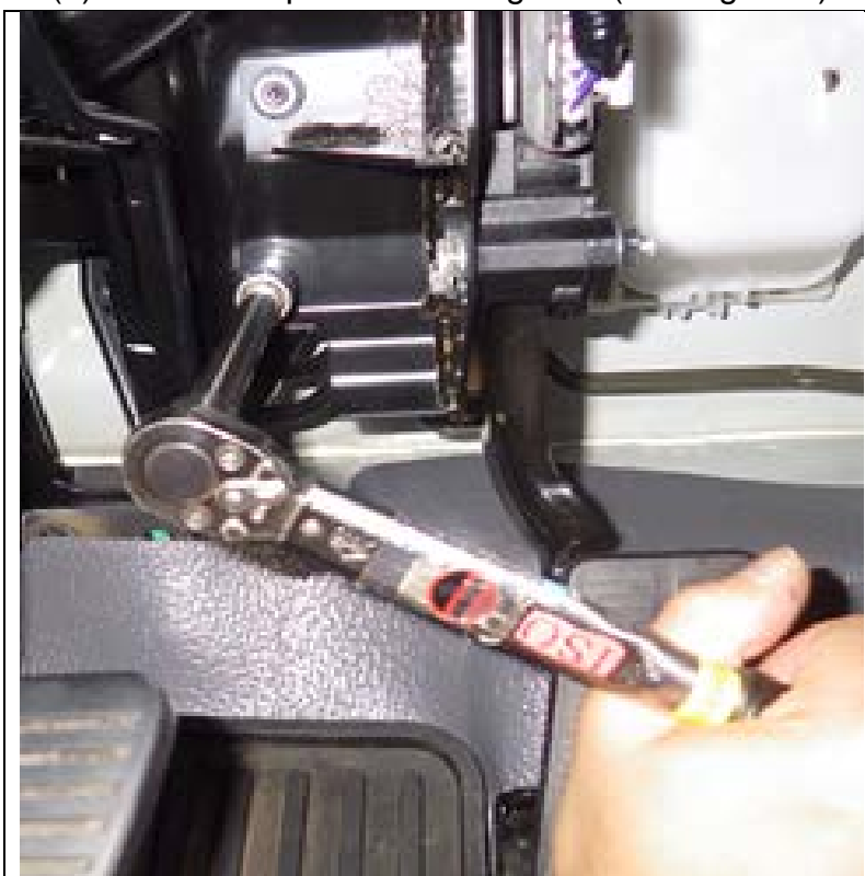
Figure 1 – Tighten Accelerator Pedal
