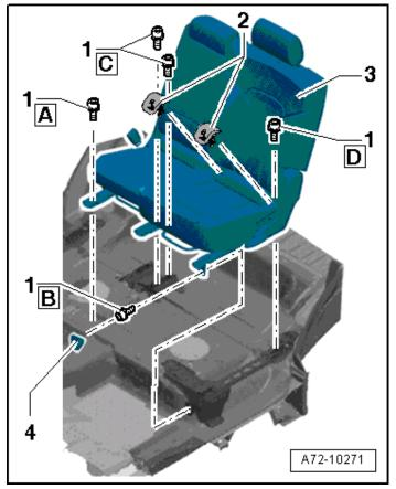
Remove the seat rail stop bolts <2> (if required).
