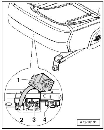
Reinstall seat rail cover trim <1> onto seat frame
