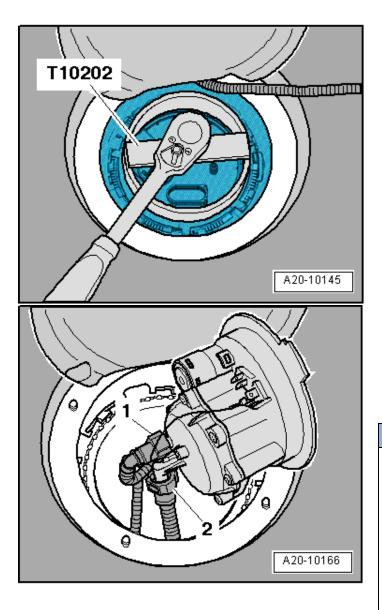
Using Fuel Sending Unit wrench -T10202-, remove the locking ring from the fuel pump flange by turning counterclockwise.
