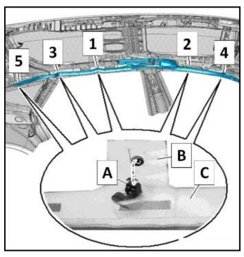
• Install the clips for the head curtain airbag in sequence <1, 2, 3, 4, 5> and ensure that each clip engages audibly into the body.
