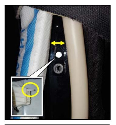
When installing the upper A-pillar trim, ensure the locating hole for the A-pillar locating pin <circle> is not covered by the head curtain airbag.
