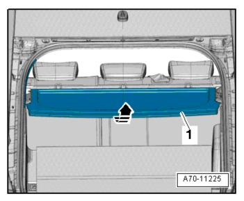
Pull the rear shelf front section <1> out toward the rear <arrow> and remove.
