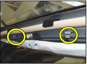
Remove and discard clamps <circles> using Omega Clip Tool -T40280- (or equivalent).
