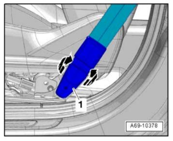
Install the belt end fitting over the pin on the seat frame and pull up on the belt end fitting until the lock audibly engages.
