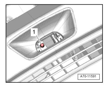
• Remove the screw <1> from the instrument panel cover.
