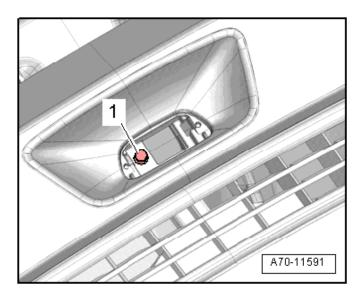
Install screw <1> and torque to 1.5 Nm.
