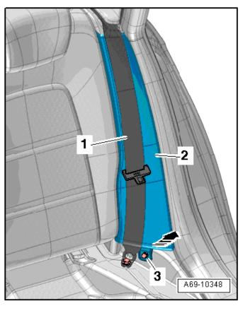
Install side cushion <2> and torque bolt <3> to 9 Nm.
