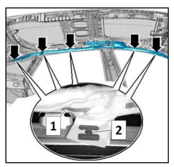
Working from outside of the vehicle, remove the clips <arrows> from the head curtain airbag
