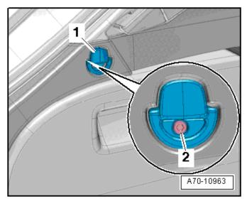
• Remove the bolt <2> and the coat hooks <1>.
