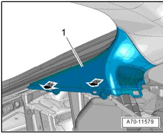
• Unclip the D-pillar trim panel <1> using the Trim Removal Wedge -3409- <arrows> and remove.
