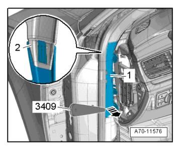
Unclip the gap cover <1> from the lower A-pillar using the Trim Removal Wedge -3409-<arrow> and remove it downward from the top of the A-pillar trim panel <2>.
