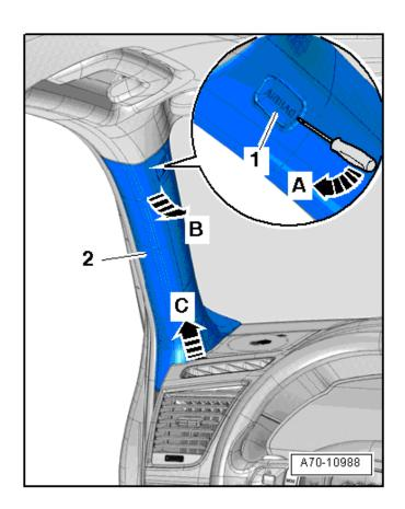
Pry out the expanding cover <1> with the "AIRBAG" symbol with a screwdriver <arrow A> and remove the screw behind the cover.
