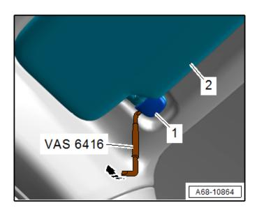
Unclip the sun visor mount expanding cap <1>
