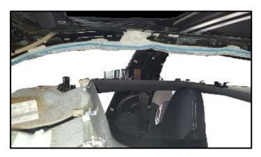
Unwrap the head curtain airbag, making sure the blue strip is visible along the entire length. This will ensure that the head curtain airbag is not twisted.
