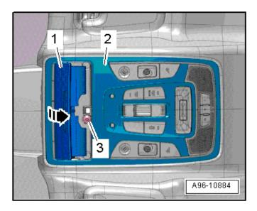
• Connect and install front roof module <2> and torque bolt <3> to 2 Nm.
