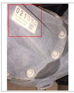
If <u>less</u> than 2.0 liters of oil was removed from the differential, a new differential carrier is required. There are two different carriers available, depending on the axle ratio. To order the correct differential carrier, you first must identify the axle ratio.
