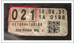
b. The numbers in the upper left hand corner of the label will identify the axle ratio.
