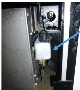
Kneeling Module behind air dryer, curbside.
