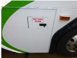
Air tank drain valve access door
