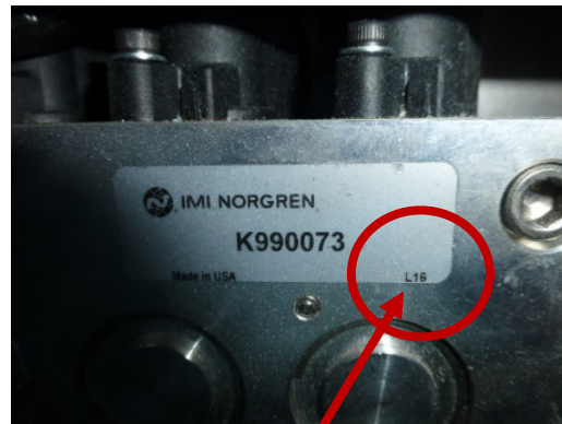
Date Code is in lower right hand corner. The date code on this module is "L16." Therefore, it does not require rework.
