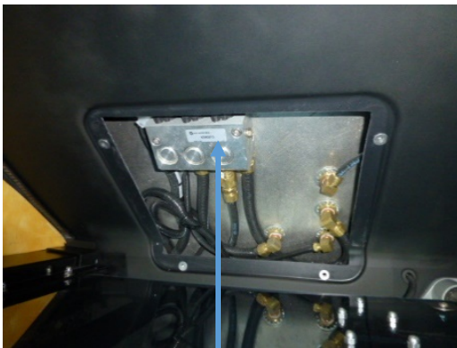
Date code on decal on face of kneeling module.
