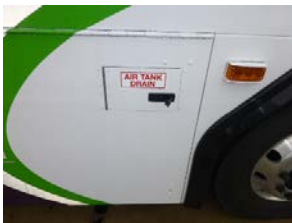
Air tank drain valve access door
