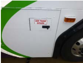
Air tank drain valve access door
