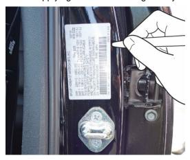
4. After the label is removed, using isopropyl alcohol on a lint free cloth, thoroughly clean the area where the new label will be attached. Make sure there is no residue from the old label, and allow the alcohol to dry.
