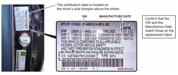
3. Use a plastic tool to remove the label. Be careful not to scratch or damage the paint.
