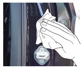
5. Apply the new certification label 10mm above the striker. Make sure the label is applied in the same orientation as the removed label.
