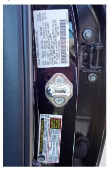
2. Confirm the VIN on the dashboard matches the VIN on the new certification label. Also, make sure the VIN and manufacture date on the new label matches the old label.
