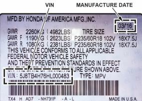
Confirm that the VIN and the Manufacture Date match those on the replacement label.  Use a plastic tool to remove the label. Be careful not to scratch or damage the paint. NOTE: Applying heat with a heat gun may make the label easier to remove.
