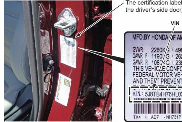
The certification label is located on the driver's side doorjam below the striker.
