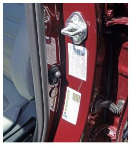
2. Confirm the VIN on the dashboard matches the VIN on the new certification label. Also, make sure the VIN and manufacture date on the new label matches the old label.
