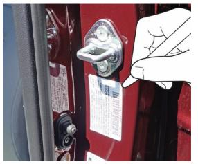
4. After the label is removed, using isopropyl alcohol on a lint free cloth, thoroughly clean the area where the new label will be attached. Make sure there is no residue from the old label, and allow the alcohol to dry.
