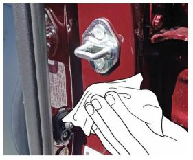
5. Apply the new certification label 10 mm below the striker. Make sure the label is applied in the same orientation as the removed label.
