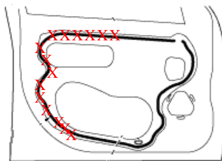
Left Front Door Film Peeling Area
