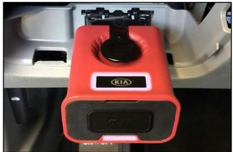
8. Confirm communication with VCI (F) and then configure the vehicle (G) using the **AUTO VIN** (H) feature.
