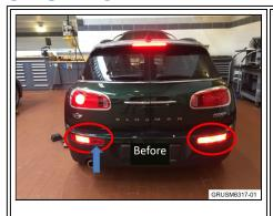
With the Clubman doors closed, activate the brake lights and pay attention to the lower lights that are located in the rear bumper trim. Both light elements will
