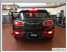
After programming is completed check the function of the brake lights in the bumper. Refer to picture. Only the outboard brake light will be on when the brakes are applied with the Clubman door closed. Only the outboard brake light will be on when either directional is turned on.
