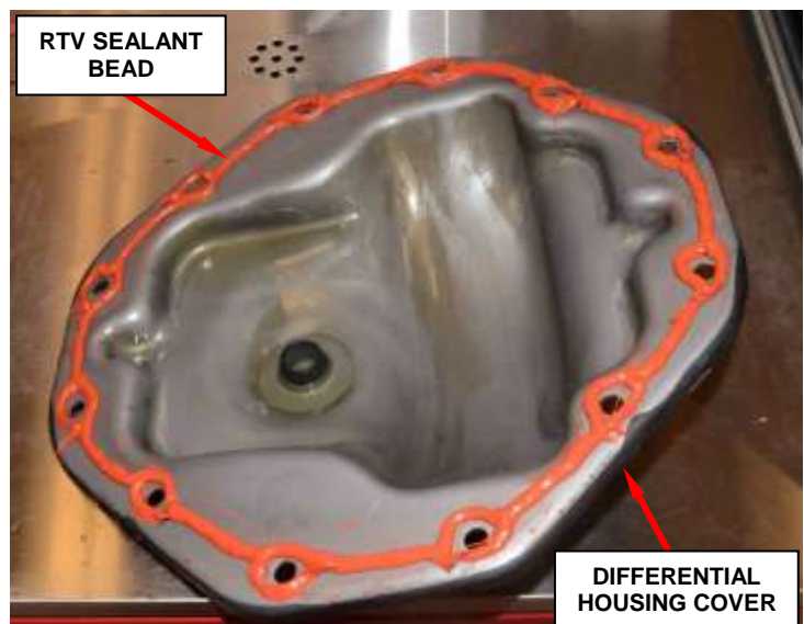
Figure 11 – Apply Mopar Axle RTV Sealant
