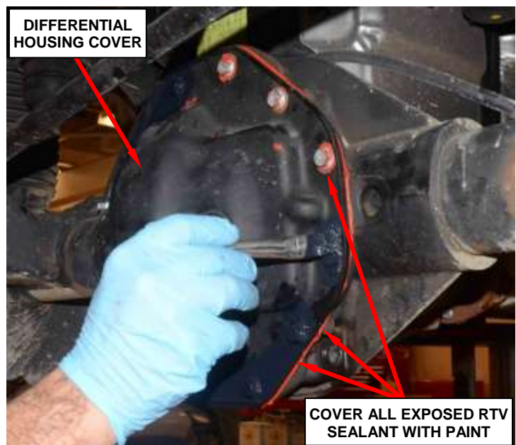
Figure 13 – Apply Black Paint to Exposed RTV Sealant
