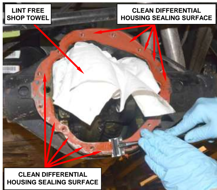
Figure 10 – Clean Differential Housing Sealing Surface
