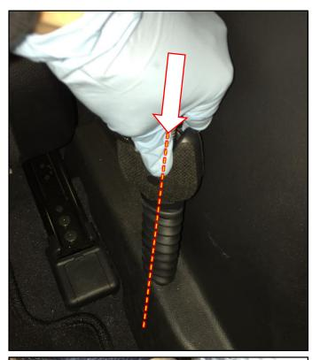
Visually inspect the center hole (F) on the outboard side of the linkage element to 5. confirm that it is fully locked.
