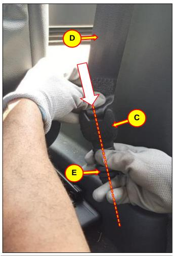
Pull the linkage element up in order to verify that it is fully locked. 3.
