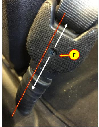
6 Move the driver seat forward, locate the driver's anchor pretensioner, and repeat Steps 2 through 5.
