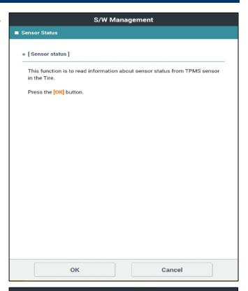
4. Read the service procedure instructions. When ready, place the TPMS tool close to the vehicle's front left TPMS sensor (no need to press the button on TPMS tool), then select **OK** on GDS.
