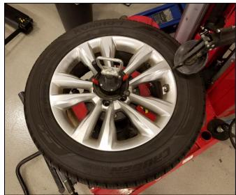
3. Depress the head to release the tire's upper bead slightly.
