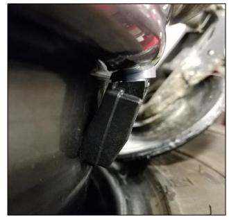
8. Remove the valve core from the new TPMS sensor.
