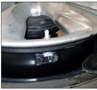
6. Remove the TPMS sensor with a deep socket and ratchet.
