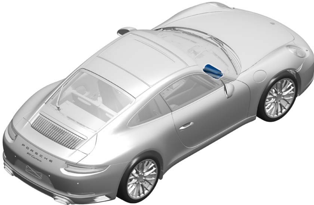
Installation position of passenger's airbag unit
