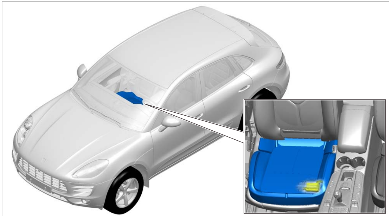
Installation position of seat occupancy detection system for passenger seat
