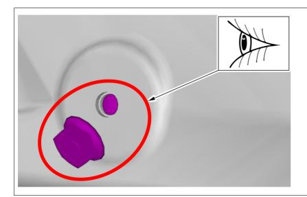
If the result of the checking procedure is not OK, the broken bolt must be replaced with a new bolt.
