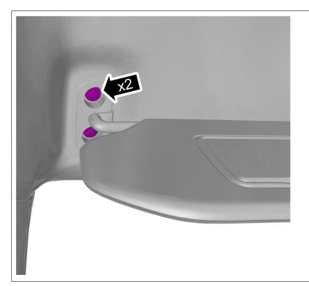
Remove the screws. On both sides.
