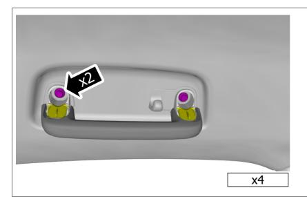
Remove the screws. On both sides.
