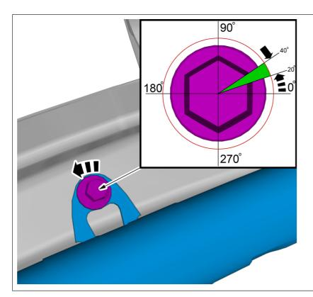
Warning! Loosen the screw between 20-40 degrees.
