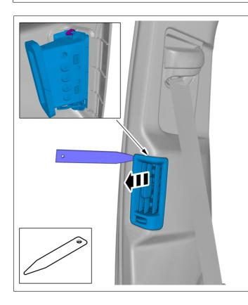
Remove the marked part. On both sides.
