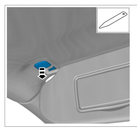
Remove the marked part. On both sides.
