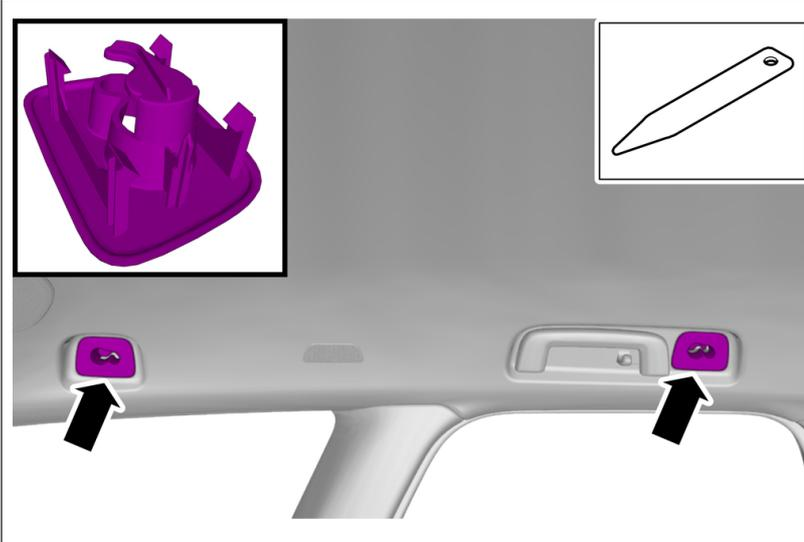
Remove the fasteners.
