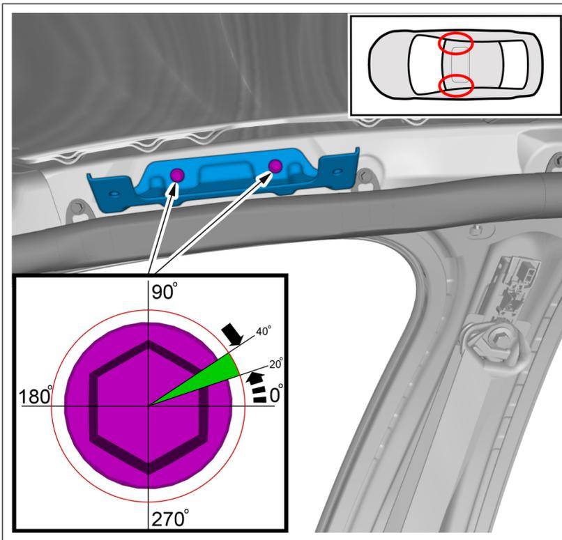
**Warning!** Loosen the screw between 20-40 degrees.
