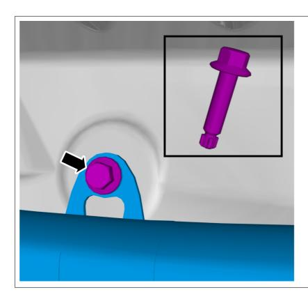
Install 22 New Inflatable Curtain bolts. Torque to 6 Nm
