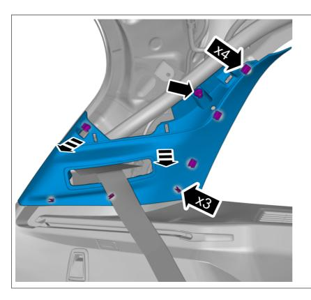
Remove the nut. Remove the panel. On both sides.
