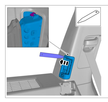
Remove the marked part. On both sides.
