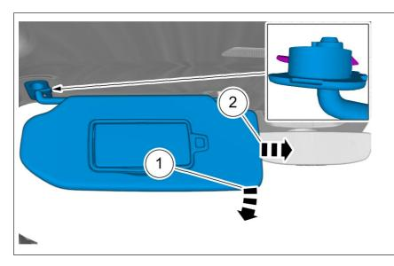
Remove the part carefully Fold marked part to one side. On both sides.
