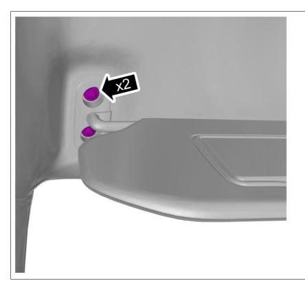
Remove the screws. On both sides.
