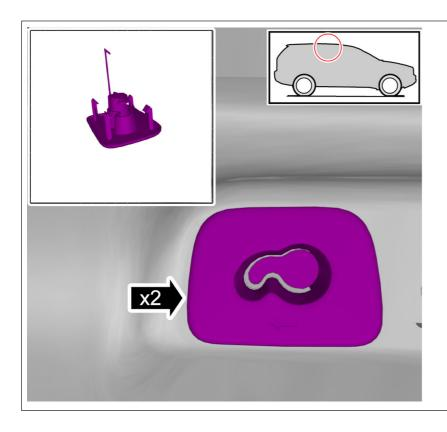
Remove the fasteners. On both sides.
