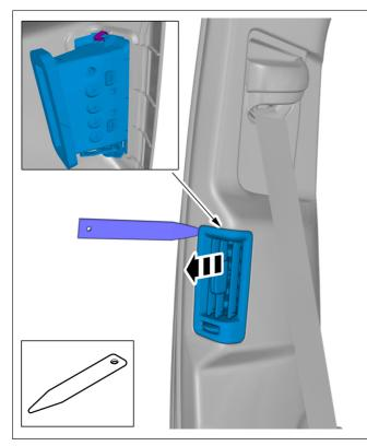
Remove the marked part. On both sides.
