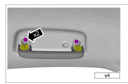
Remove the screws. On both sides.
