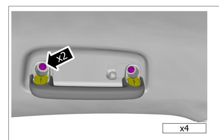
Remove the screws. On both sides.
