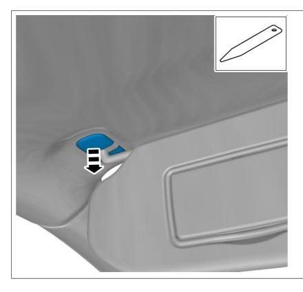
Remove the marked part. On both sides.
