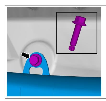
Install 16 New Inflatable Curtain bolts. Torque to 6 Nm
