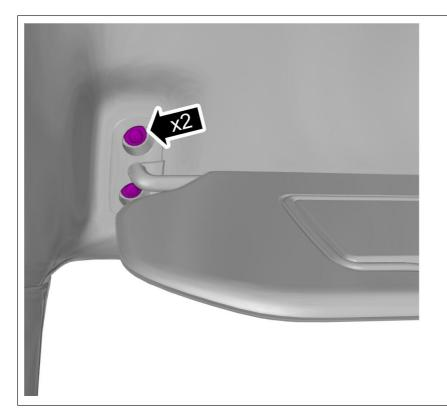
Remove the screws. On both sides.
