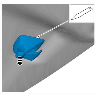
Remove the marked part. On both sides.
