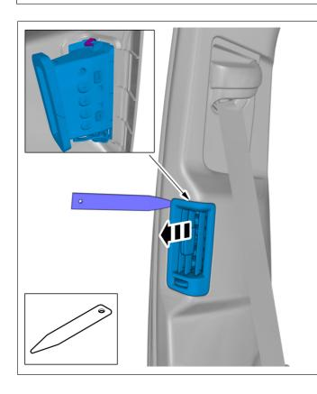
Remove the marked part. On both sides.
