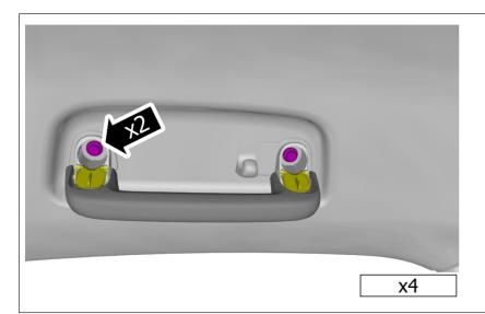
Remove the screws. On both sides.
