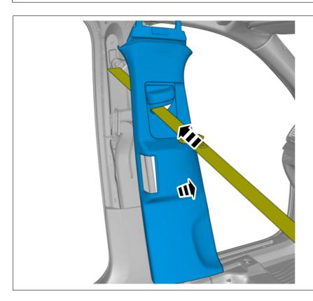
Fold marked part to one side. On both sides.
