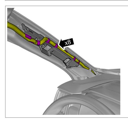
Loosen the wiring harness or move it to the side.
