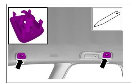
Remove the fasteners. On both sides.
