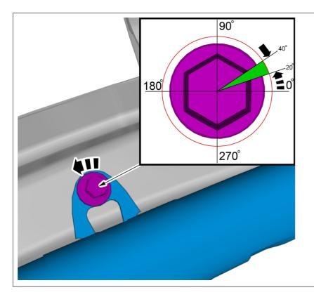
Warning! Loosen the screw between 20-40 degrees.
