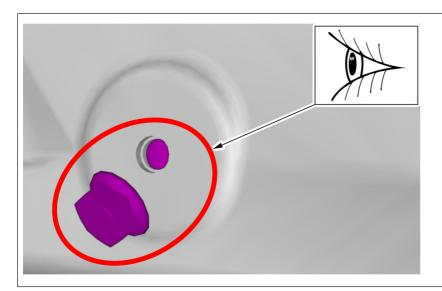
If the result of the checking procedure is not OK, the broken bolt must be replaced with a new bolt.
