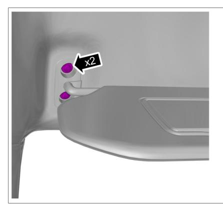
Remove the screws. On both sides.
