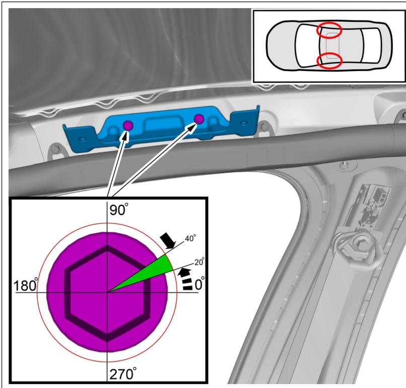
**Warning!** Loosen the screw between 20-40 degrees.
