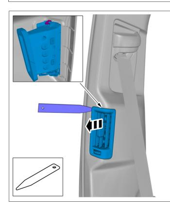
Remove the marked part. On both sides.
