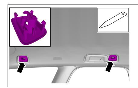
Remove the fasteners. On both sides.
