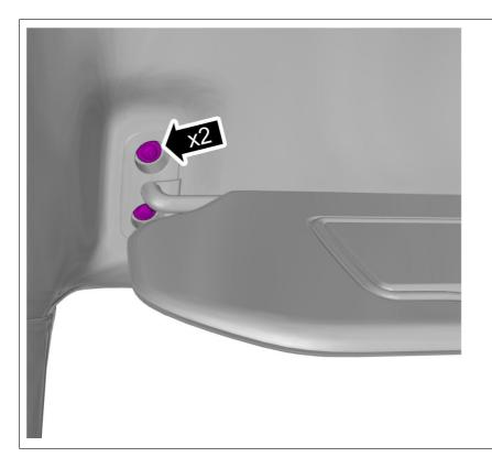
Remove the screws. On both sides.
