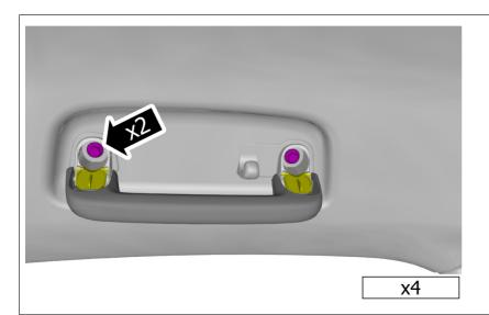
Remove the screws. On both sides.
