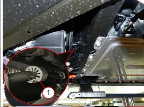
8. Secure the new abrasion protection (1) on a suitable position on the tank ventilation line, so that it protects from any contact between the tank ventilation line and the fuel feed line (2).
