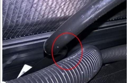
4. This example shows slight damage which is acceptable. Proceed to step 6.
