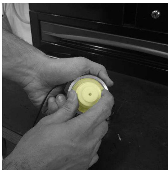
73. Assembling the fuel tank cap.
