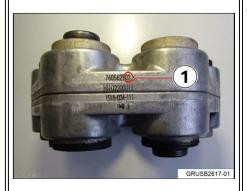
NOTE: If the revision number cannot be read, replace the flexible disc.
