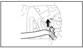
d) Clip the wire harness retaining clip into the top of the *NEW* side stay.
