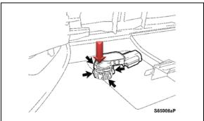
b) While depressing the 4 retaining claws, push the end of the sensor and gently roll the sensor through the bumper pad.
