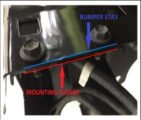
c) Align the *NEW* side stay so that the edge is parallel with the mounting flange from the hitch/draw bar.
