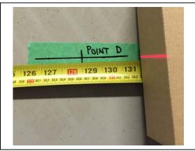
e) Mark a point 128 ½" (3264mm) from the vehicle centerline (Point C). Label this Point D.
