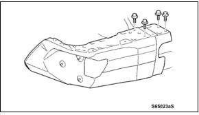
b) Reinstall the 4 bolts on the top of the *NEW* side stay, but **do not tighten**.
