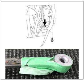
c) Reinstall the 2 bolts on the bottom of the side stay. The rearmost bolt will require a *NEW* nut as shown. Do not tighten the bolts.
