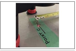
i) Set the end of the tape measure on the vehicle centerline at Point C.
