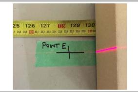
j) Mark a point 128 ½" (3264mm) from the vehicle centerline (Point C). Label this Point E.
