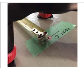
d) Set the tape measure on the vehicle centerline at Point C.
