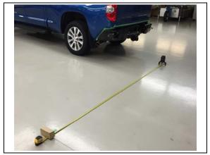
h) Lay a tape measure along the laser line. Extend the tape more than 135" (3,430 mm).
