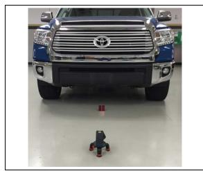
f) Rotate the laser level clockwise and counter clockwise until the vertical beam is centered on the Toyota logo as shown in Step 1e above.
