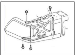
b) Start the 4 *NEW* bolts as indicated, but **do not tighten**. Do not install a bolt in the 5<sup>th</sup> bolt hole at this time.
