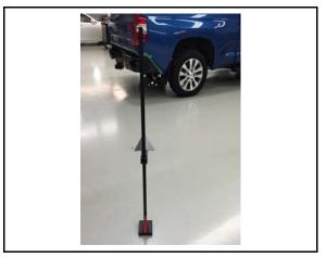
b) Aim the reflector toward the RH Blind Spot Monitor Sensor.
