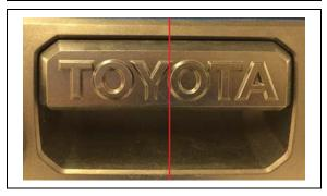
b) The "TOYOTA" label on tailgate release handle will be the reference point for the rear centerline, midway between the "Y" and the "O".
