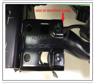
b) Use the edge of the mounting flange on the hitch / reinforcement bar as a reference for proper alignment of side stay.
