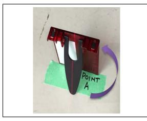
k) Rotate the laser target 180 degrees, so that it faces the rear of the vehicle. Be sure to line up the centerline of the target with Point A.
