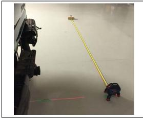
c) Lay a tape measure along the laser line that is a 90 degree right angle to the vehicle centerline. Extend the tape more than 135" (3,430 mm)
