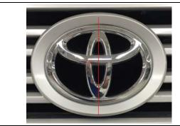
e) The centerline of the Toyota emblem in the grill will be the reference for vehicle front center point.
