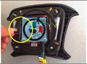
3. Place the horn contact plate on the new air bag module and plug in the connector.
