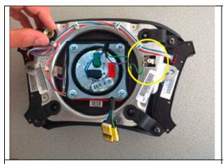
5. Plug in the connector for the grounding cable and secure the horn ring with the four Torx nuts.
