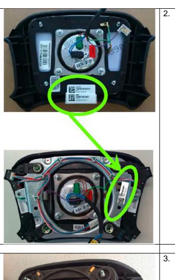
2. Prepare the new air bag module and pull off one of the two labels with the barcode and serial number of the air bag module. This must be stuck onto the horn ring after installation.
