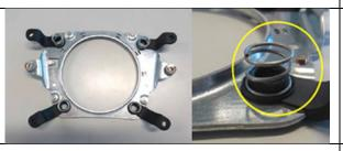
4. Place the horn ring on the air bag module. Make sure the springs are seated correctly.
