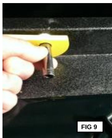
FIG 9: Install the 6mm "keps nut" by hand until snug.
