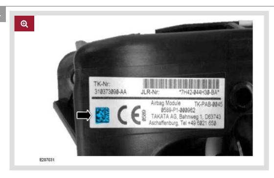
Locate the QR code on the NEW passenger airbag module label.
