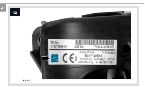
Locate the QR code on the NEW passenger airbag module label.
