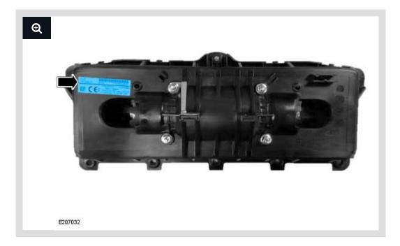
Locate the label on the NEW passenger airbag module.
