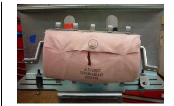
b) Mount the airbag to the mouting bracket as shown.
