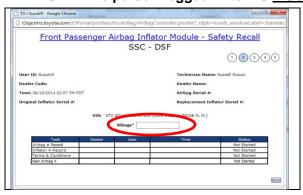
e) Record the vehicle mileage into the serial number recording application.
