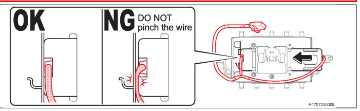
d) Insert the inflator with the correct orientation as shown in the illustration.
