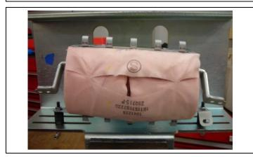
b) Mount the airbag to the mouting bracket as shown.
