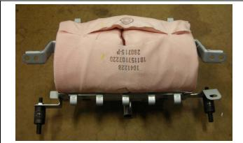
a) Mount the adaptors (579943-3R3) to the airbag as shown.
