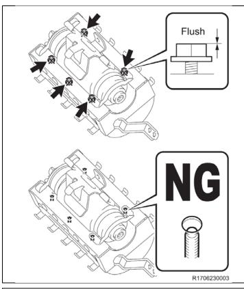
c) Loosen the 5 nuts until each nut is flush with the top of the stud as shown.
