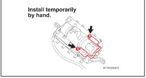
e) Temporarily install a **NEW** plate and airbag inflator with the 2 **NEW** self-locking nuts.
