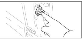
If the anti-static kit is not available, before starting work and periodically while working on the vehicle, touch a metallic part of the vehicle to discharge static electricity in the body.
