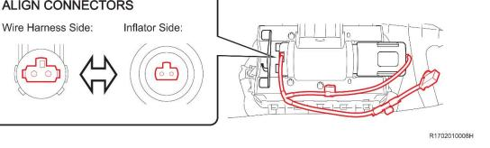
a) Fully insert the inflator and ensure that the inflator is correctly orented as shown. NOTE: DO NOT pinch the wiring between the bracket and the inflator.
