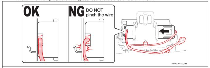
NOTE: Ensure the inflator is correctly oriented.
