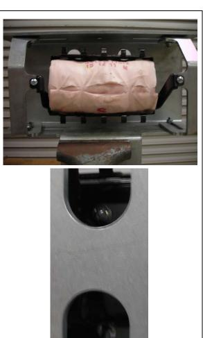
f) Mount the airbag into the mounting bracket as shown.
