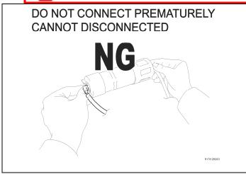
NOTE: Once connected the inflator harness cannot be disconnected without damaging the connector, and would require that the inflator and harness be replaced.
