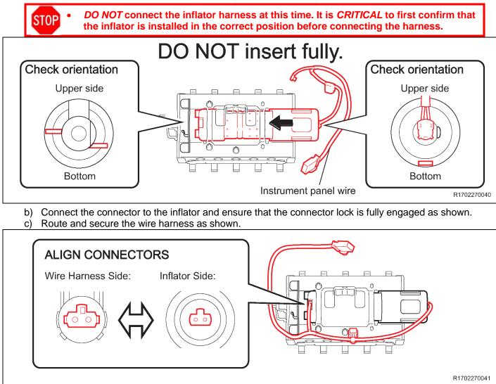
d) Fully insert the inflator and ensure that the inflator is correctly orented as shown. **NOTE: DO NOT pinch the wiring between the bracket and the inflator.**
