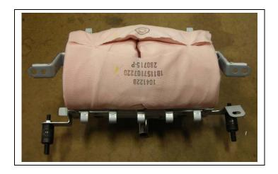
b) Mount the adaptors (579943-3R3) to the airbag as shown.
