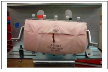
c) Mount the airbag to the mouting bracket as shown.
