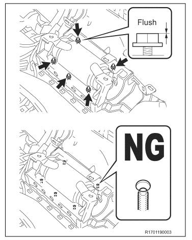
d) Loosen the 5 nuts until each nut is flush with the top of the stud as shown.
