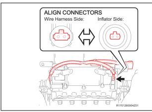
m) Connect the connector and the secondary lock
