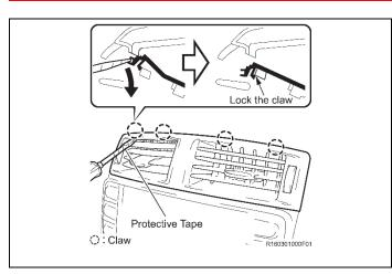
Removing the No. 3 air register
